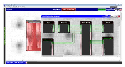
Besides all the parameter, preset, and control programming work that would normally be done, our focus here is the preparation for adding a 2x2 I/O - Rio R22 Dante interface to the input side of our processor and a 4x4 I/O - Rio R44 Dante interface to the output side of our Neutrino-N processor.
