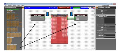
Next, as indicated by the blue arrows above, you wire them to the processor modules applicable Network Inputs and Network Outputs and to complete the procedure, we need to provide Source Labels for the Virtual Transmitter on the input side and **Destination Labels** for the *Virtual Receiver* on the output side.
