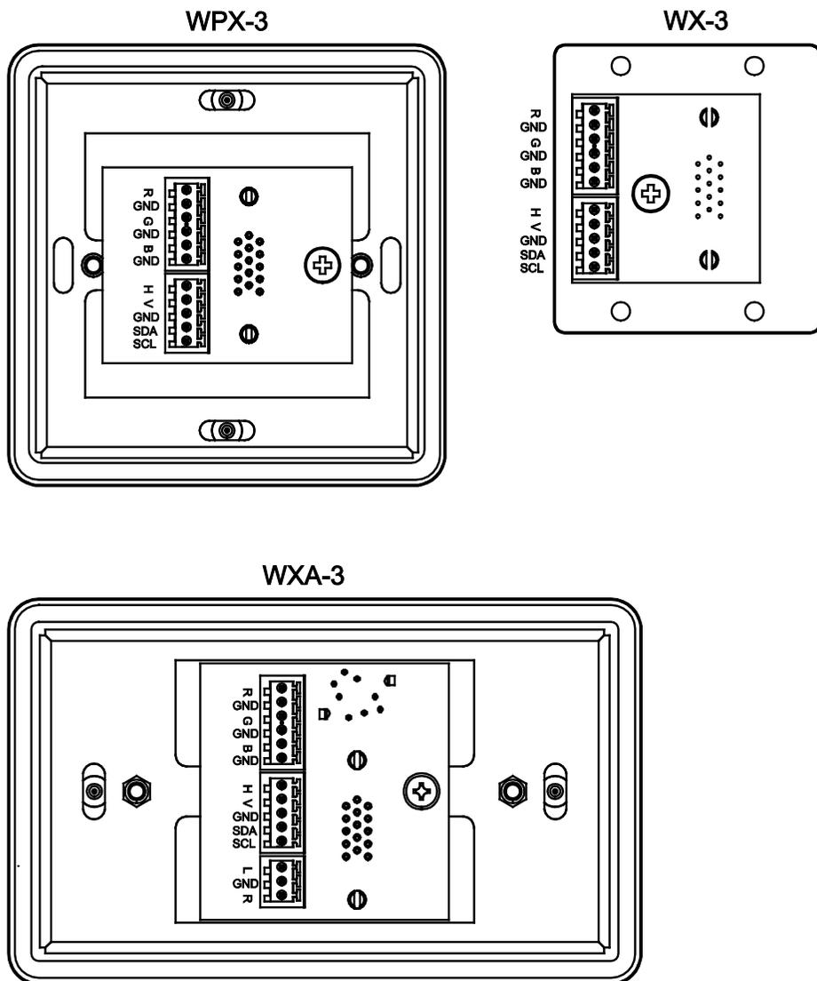
Figure 4: Pinout on Rear Panel
