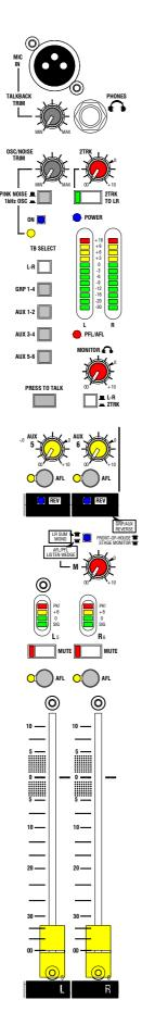
**AUX 5 and 6 Masters** These function in the same way as described for auxes 1 to 4. The REV switch reverses the AUX5 mix with L, and AUX6 mix with R for operation in monitor mode. When selected, the aux signals are presented to the L and R XLR outputs complete with their inserts. The LR mix swaps on to the Aux TRS jack outputs. Note that the LR mix always feeds the matrix regardless of mode selected.
