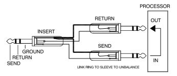
**DIRECT OUTPUT** The mic/line channel direct output is available on an impedance balanced TRS jack. It is a line level signal operating at 0dBu. The source is set using an internal option jumper for each channel. The factory default setting is pre-fade (following the pre/post-EQ setting). This may be changed to post-fade if preferred.
