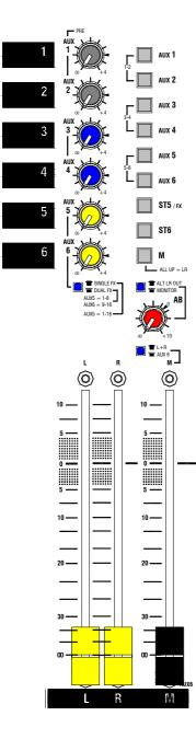
**AUX MASTERS** Each aux mix has a master level control that adjusts the output level to match external equipment, or to trim the monitor, effect or other send without affecting the mix balance. Up to +4dB boost is available above the normal 0dB position.
