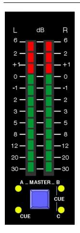
This is an easy-to-read 2- x 12-segment LED display. The signal on the VU-meters is the signal on the headphones output (master A, master B, master C or the CUE signal).
