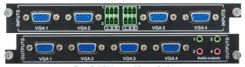
**Figure 8 - VGA Input and Output Cards**
