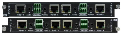
Figure 11 - HDBT Input and Output Cards
