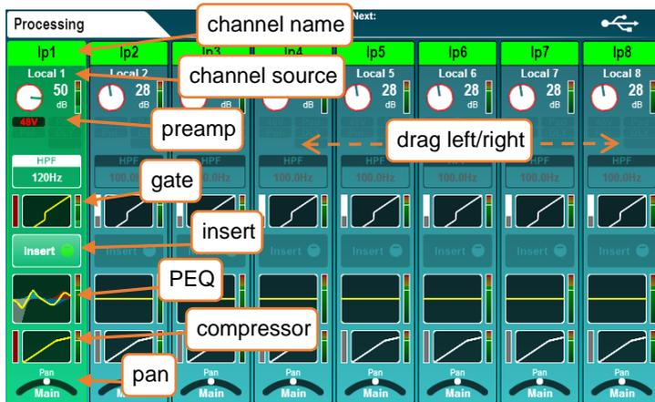
This gives the processing overview for 8 channels at once, with the selected channel highlighted. The view will automatically change if a channel is selected which is out of view, though you can also touch and drag to see all channels for the current layer. The selected mix channel is displayed to the far right.
