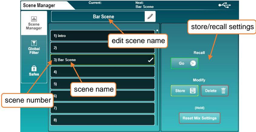
To store all current mix settings in a new slot, touch any empty slot then:
