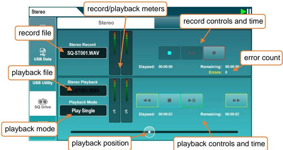
The top half of the screen is for recording and the bottom half is for playback.
