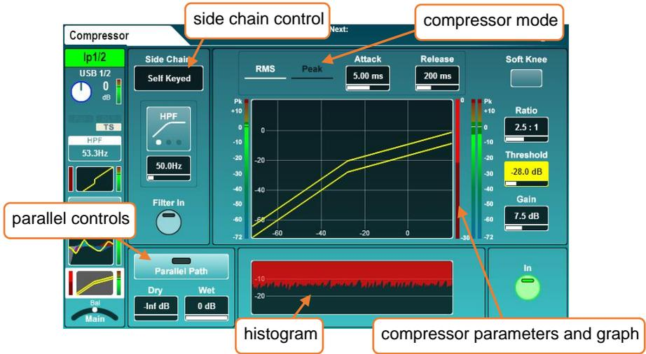
Switch the Compressor in or out using either the on-screen 'In' button or the physical Compressor 'In' key (to the left of the dedicated Compressor threshold rotary).
