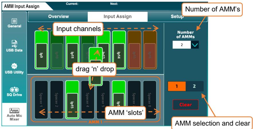
The top part of the screen shows the available input channels and at the bottom are available AMM slots.
