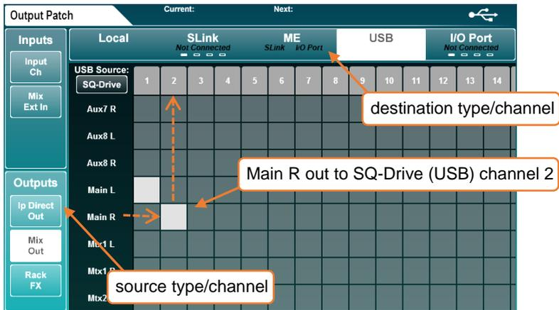
USB patching is for SQ-Drive or USB-B streaming connections.
