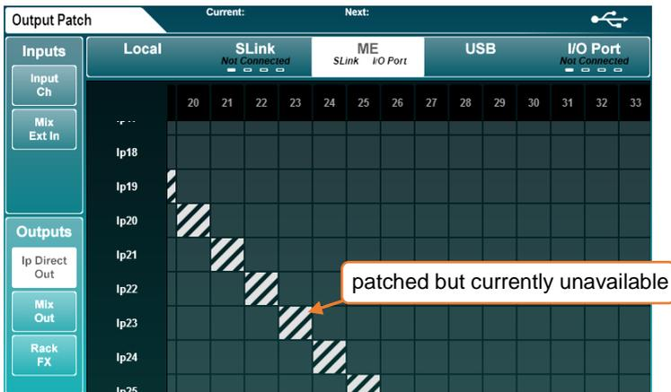
The ME patching is applied to either the SLink port, the I/O Port, or both.
