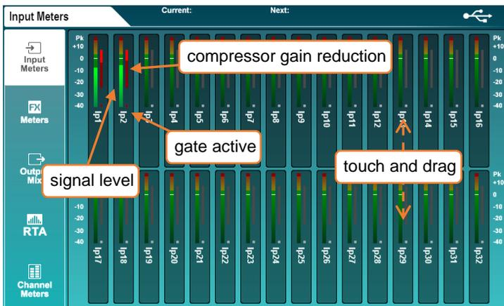
The first three tabs on the **'Meters'** screen show **'Input Meters'**, **'FX Meters'** and **'Output Meters'**.
