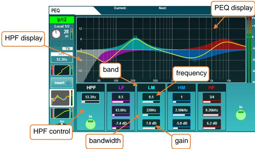
**HPF** - In order of processing, the High Pass Filter (HPF) is located post-preamp (as in the channel overview). It is displayed in the EQ screen for convenience.
