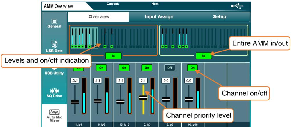
The top part of the screen displays an overview of all AMM slots, with the metering showing gain being applied to channels and indication of whether or not channels have AMM switched on.
