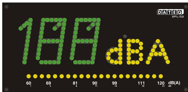
The SPL-D2 unit is a separate sound-level meter. Besides it can be linked to the SPL5 limiter. The unit is a large LED display, showing the actual sound-pressure level. The LED-bar at the bottom can be configured as a VU-meter, or a reduction meter (when linked to the SPL5).
