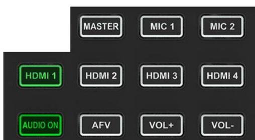
After pressing one Part A button, the indicator of button in Part B is on in green means the corresponding audio function is on. When the indicator is off means the corresponding function is off.
