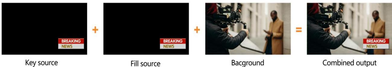
Downstream keys are the last layers of keying, so they overlay all video switched to the main program output. They operate independently to what's selected as the "background", whatever you place on a Downstream key is going to stay on screen, no matter what you are doing with your transitions. Downstream key is ideal for bringing animated bugs or logos on screen.
