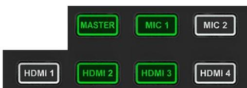
When the indicator of button in Part A is on in green means the corresponding audio is on. When the indicator is off means the corresponding audio is off.
