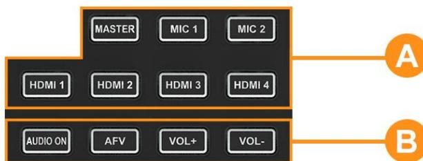
Part A is for selecting one audio to be configured, including Master, MIC 1, MIC 2, HDMI 1, HDMI 2, HDMI 3 and HDMI 4.
