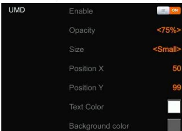
The UMD string content for 4 HDMI inputs can be set from menu. User can rename the UMD content for each window by using a virtual keyboard and rotary button. It supports input max 10 characters for the UMD content. Below image as an example, rename the HDMI 1 to CAM1.
