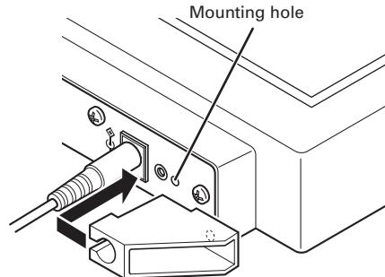
3. Fix the holder to the RC-F400S using the included screw.
