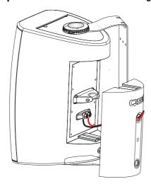
**5-** Strip the speaker wiring ends and connect the wires. If using the YM-8, connect the wires directly to the binding posts. If using the YM-8T, connect the 70V/100V terminals in the cover assembly.
