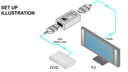
The **PT-2HDMI** input is connected via a long male-to-male HDMI cable (not provided) to an HDMI source, such as a DVD player or a satellite set top box.
