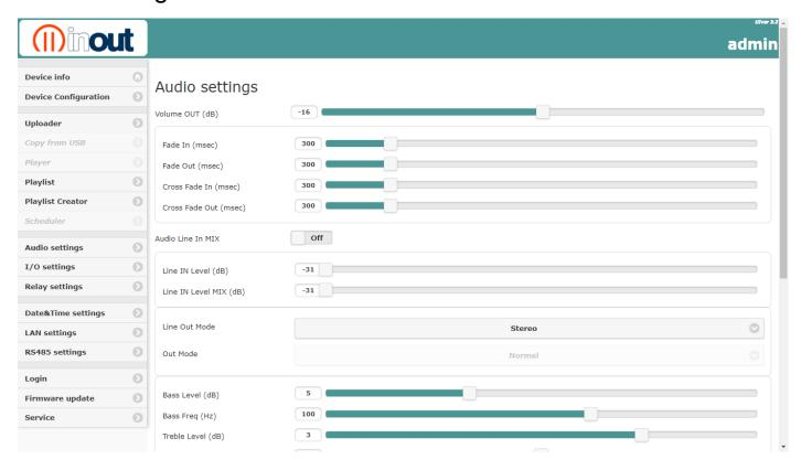
Volume out: level preamplified and amplified audio output
