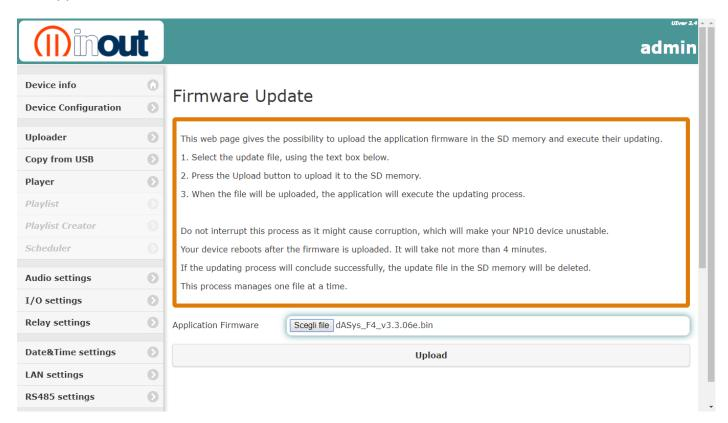
The process uploads the file in the SD card memory, inside the directory "updates", check the file integrity using the CRC info and then decrypt the data and write them in the Flash area. Instead, in the App, after the integrity check will recall a sw reset, in order to execute the bootloader that will find the file in the "updates" directory.
