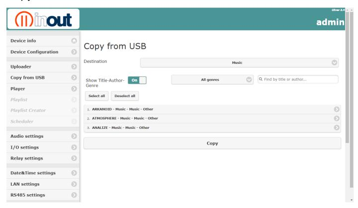
To copy files into NP2/NP5, insert USB pen drive, select the audio files, select dir/folder destination and press Copy to transfer files into microSD storage.
