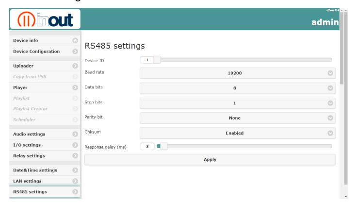
**Device ID:** Address NP2/NP5 in the 485 bus. This address **MUST** be univocal, two devices with the same address can not co-exist on the same bus.
