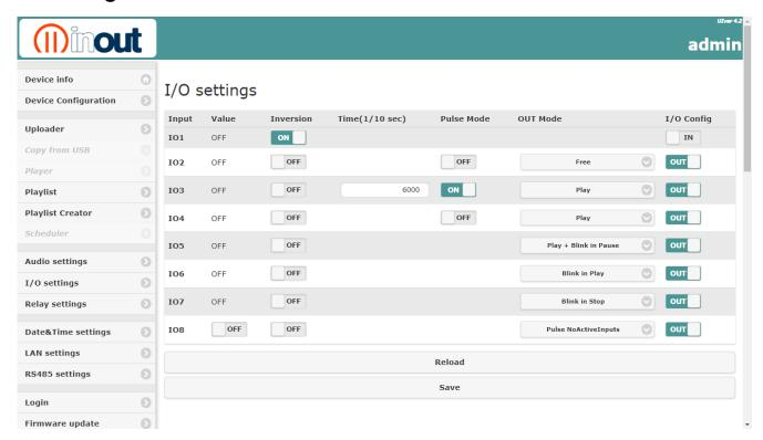
I/O Config: Setting logic port input or output
