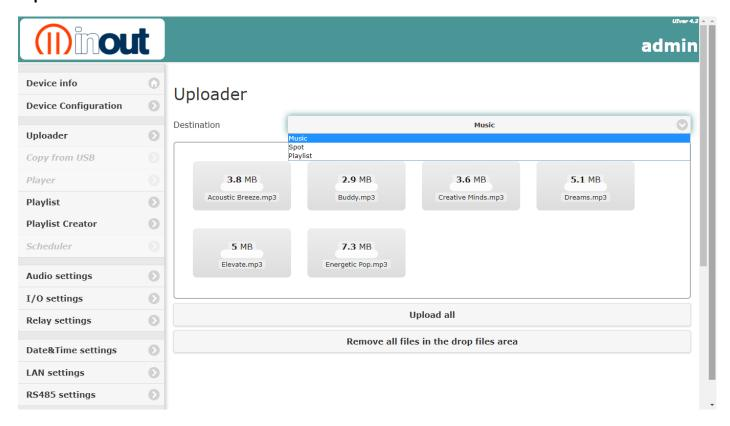
To upload files into NP2/NP5, select the audio files on your computer/device, select dir/folder destination and press Upload all to copy into microSD storage.
