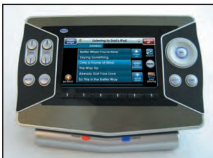
Red indicates charging, Blue that the remote is fully charged.
