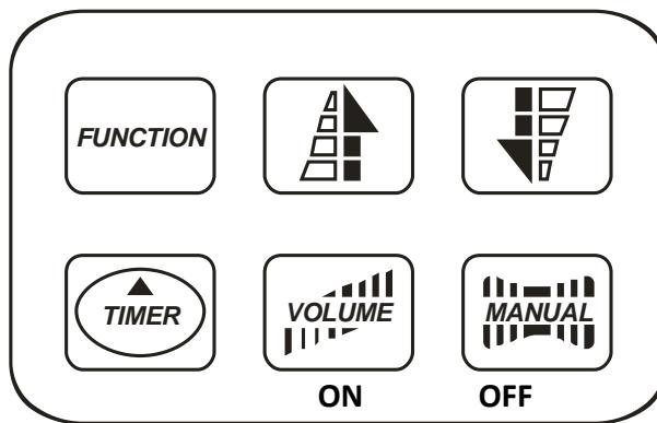
The built-in control panel of the machine features an LCD panel displaying all operation statuses of the fog machine. The control panel allows the user to customize fog machine functions by adjusting the fogging duration, interval, and volume as well as the DMX address and the pump sensor. There are six buttons on the control board. All current operating
