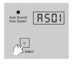
Tap Mode Select button until LED under Auto Sound/ Auto Speed is lit and the LED display reads "AS01", this unit is in Auto Sound mode.
