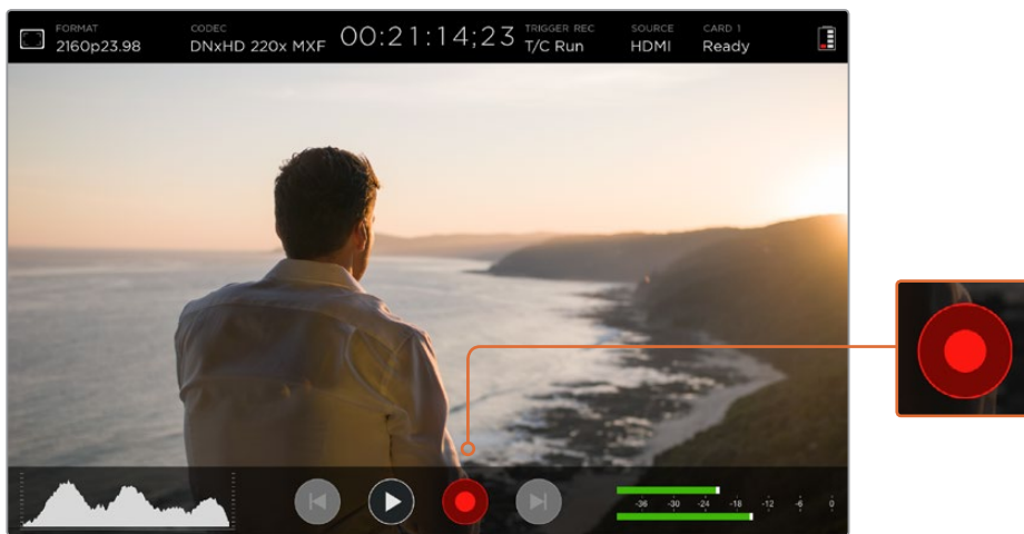
To start recording, simply swipe the touchscreen up or down to reveal the on screen meters, then tap the 'record' icon. Tap again to stop recording.
