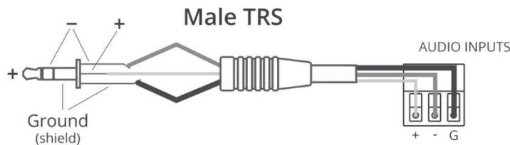
Figure 5: Connecting a Balanced 6.5mm Phone Jack
