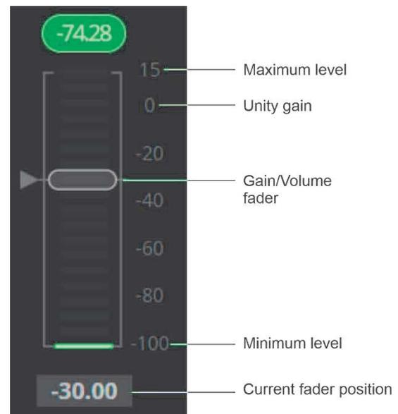
Figure 24: Channel Fader
