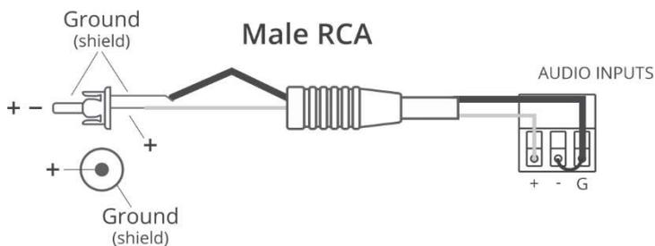
Figure 6: Connecting an Unbalanced RCA Input
