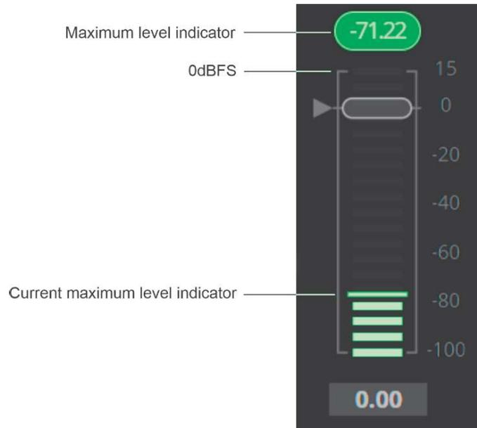
Figure 23: Level Measurement Indicators
