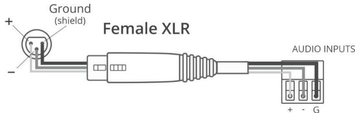
Figure 4: Connecting a Balanced XLR Input
