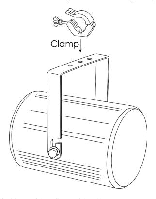
The PSB-510M can be mounted to any kind of truss with a clamp.
