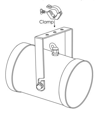
The PSB-510P can be mounted to any kind of truss with a clamp.
