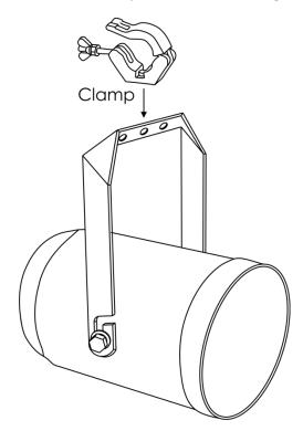
The PSU-620P can be mounted to any kind of truss with a clamp.
