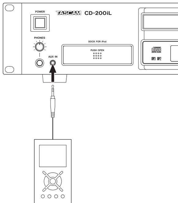
By connecting the analog output (line out or headphones jack) of another type of audio player or an iPod/iPhone that does not have a Lightning or Dock connector to the **AUX IN** jack on the front of this unit, you can output sound from these audio players through the output jacks of this unit. Since the **AUX IN** jack does not have an input level adjustment, adjust the output level from the connected device.
