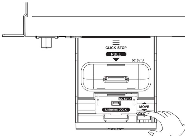
4. Insert a dock adapter that is suitable for your iPod or iPhone with a 30-pin Dock connector into the 30-pin Dock connector section, and then connect that iPod or iPhone.
