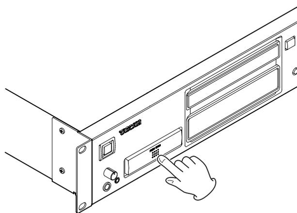
2. Pull the iPod dock out until you can use the Lightning connector and it locks. Then, raise the backstop.
