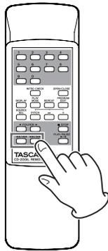
After selecting the track, press the **PLAY/PAUSE** button on the main unit or the remote control to start track playback.
