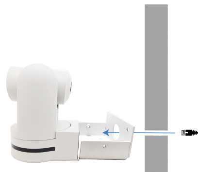
Figure 5: Connecting cables from behind the wall
