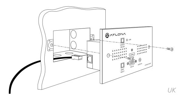
The UK wall plate screws will be the longer than the US screws. Thread the screws through the two holes in the UK wall plate and into the back box (as shown above).
