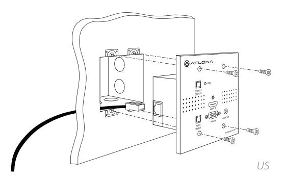
When installing the US version, use the four shorter screws. Thread the screws through the face plate into the back box (as shown above).
