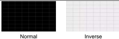
The Cross Hatch 8 pattern is a full field black & white pattern of crossing vertical and horizontal lines dividing the screen into 8 sections in each direction. This pattern is primarily used to check for color convergence and pincushion issues in projectors. There are 2 variations: Normal (white lines, black field) and Inverse (black lines, white field).
