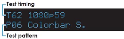
Figure 12: OLED Display – Pattern Mode with Connected Sink
