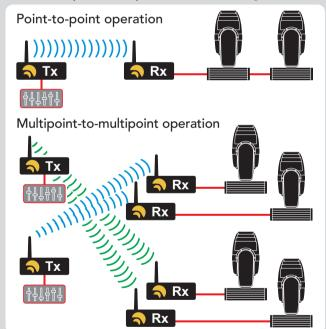
W-DMX™ is unique in its use of certain advanced radio techniques which are more often found in mobile phone and military communications. Rather than using fixed frequency channels, W-DMX™ uses adaptive frequency hopping technology (as well as TDMA and GFSK techniques) to continually check for interference and to rapidly move operation over to clear radio channels. The frequency hops occur one thousand times every second to ensure smooth, efficient and robust operation.
