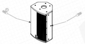
When mounting RF 10 vertically, unscrew sockets on the sides. Do not use these removed screws for mounting - proper size screws for attaching bracket are included with V10B.
