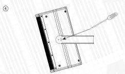
Fix loudspeaker angle with self-driving screws on both sides of the bracket. It is necessary to use these screws to keep loudspeaker from shifting angle due to weight and vibration.
