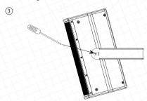
Place loudspeaker into the bracket and tighten the screws on both sides. Plug audio cables and make final angle loudspeaker adjustments.
