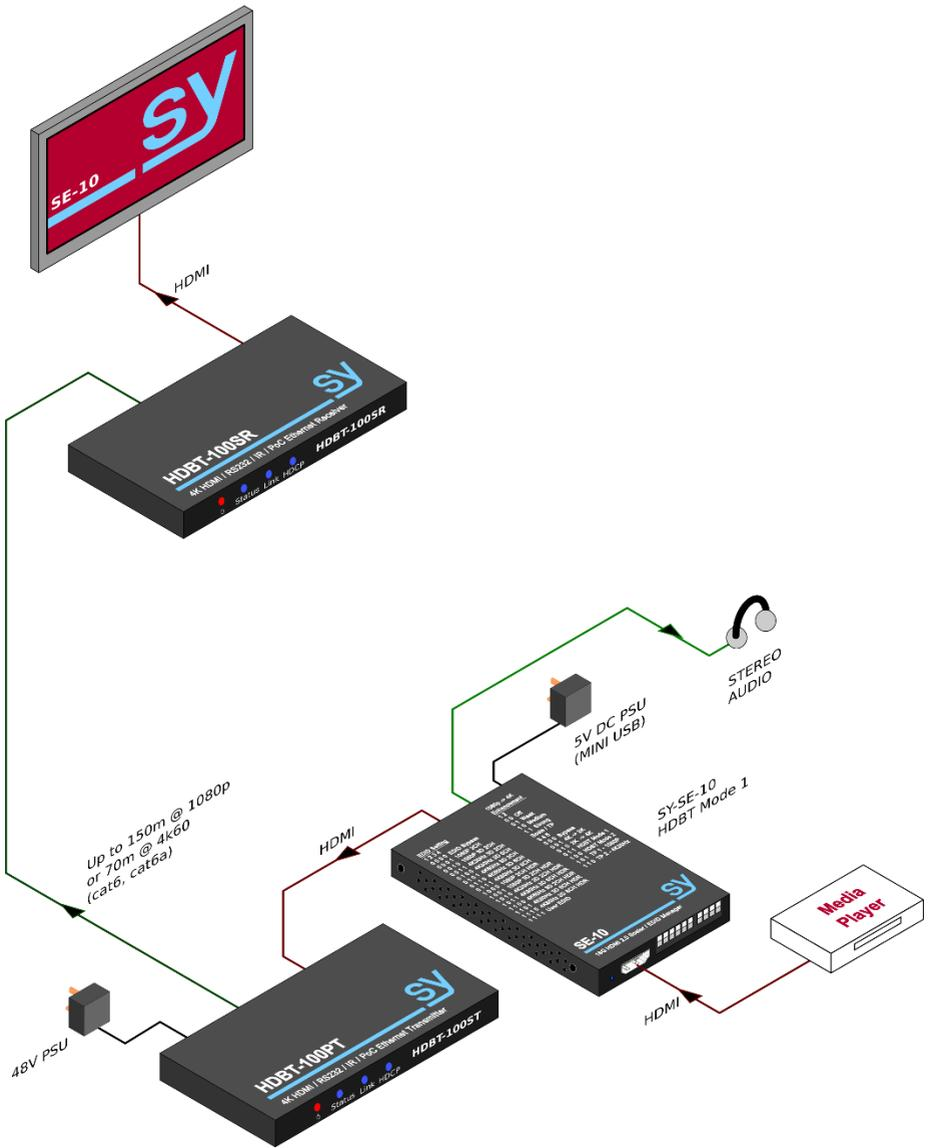
Figure 4 – Example of SE-10 with Extenders, in HDBT Mode 1 Setting
