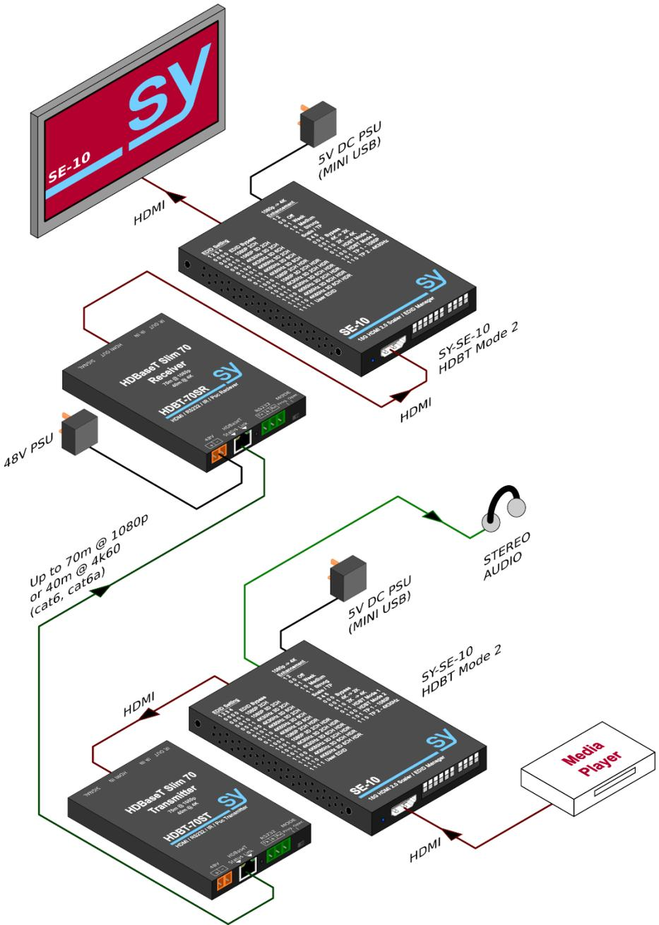
Figure 5 – Example of SE-10 with Extenders, in HDBT Mode 2 Setting
