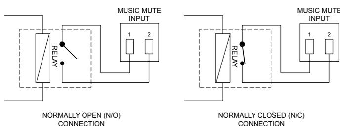
Note that any signal applied to the Facility Port – either from a remote active module, or as a hard-wired direct input, will also be muted by the action of Music Mute.
