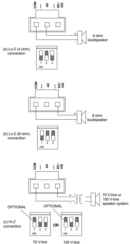
When driving 70/100 V-line loudspeaker systems there is a risk of transformer core saturation at high levels and low frequencies, which can produce distortion. To prevent this, the mixer-amplifier's output stages is provided with a 65 Hz high-pass filter, which may be enabled by setting **SPEAKER SETTINGS** switch SW1 to on (switch down).
