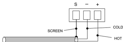
12 V phantom power is available at the mic input, and is activated by setting internal jumper J9 to the ON position. See page 25 for locations of internal jumpers. Care should be taken to ensure that phantom power is activated only when the microphone connected to the input requires it – i.e., a capacitor or electret type; other types of microphones (such as dynamic) may be damaged if a DC voltage is applied to them.
