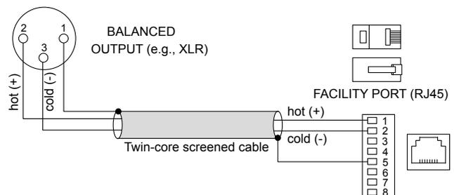
An unbalanced source may also be connected; the use of balancing transformers is recommended.
