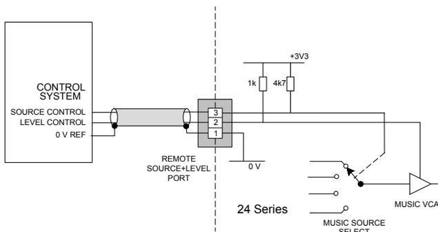
**NOTE:** If the control voltage source is not isolated from the power earth, there is a small risk of creating a 'ground loop' by linking the mixer technical ground (0 V) to the ground (0 V) of the equipment supplying the control voltages. To minimise this risk, we suggest that all pieces of equipment be in close proximity, and supplied from the same power outlet.
