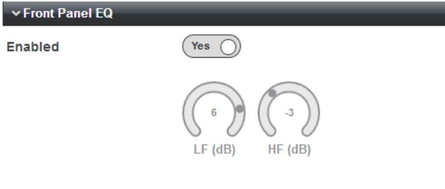
The on-screen rotary controls on this tab are not active: they are mimics of the physical front panel controls. With the **Enabled** switch set to **Yes** (the default setting), the mimics are visible (though they are always greyed out) and the physical controls themselves are enabled. Setting **Enabled** to **No** disables the controls and places the EQ section “out of circuit”, resulting in a “flat” EQ response; this will generally be desirable if the Room EQ software controls are to be used.
