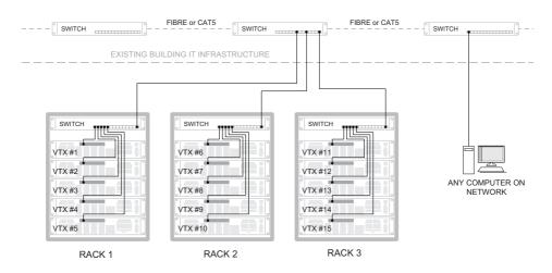
As many amplifiers and racks as required can be networked in this way, and these may, of course, be anywhere in the building. The only requirement is that each rack switch is connected to the same building network, so that all amplifiers in the system are accessible from a computer elsewhere on the network.
