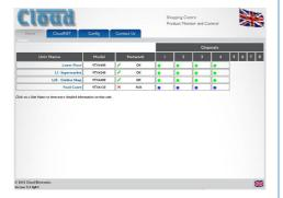
A green indicator in the Channels columns confirms that each channel of each amplifier is operating normally.
