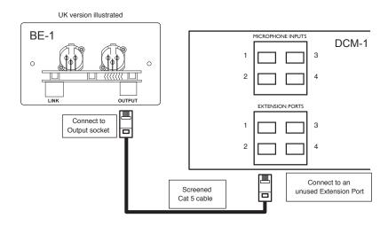
Note that all BE-Is have two RJ45 connectors, OUTPUT and LINK. On BE-I and BE-IA versions, they are both mounted on the lower PCB, with the OUTPUT connector on the right (looking at the module rear), and LINK conector on the left. On BE-IM versions, they are mounted on the upper PCB, again with the OUTPUT connector on the right.
