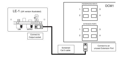
Note that all LE-1s have two RJ45 connectors, OUTPUT and LINK. These are both mounted on the lower PCB, with the OUTPUT connector on the right (looking at the module rear), and the LINK connector on the left.
