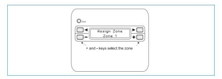
Use the + and – keys to scroll to the zone required, unless Zone I is correct. Press the ZONE button to accept the assignment (the display changes to the Set Key screen); after a few seconds, the CDR will enter normal User Mode, with the zone assignment confirmed
