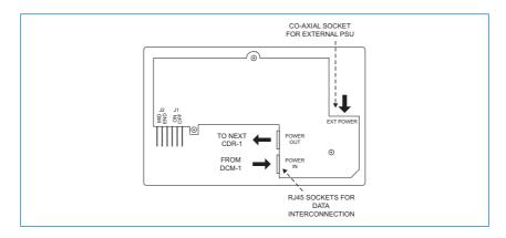
5. Check that jumper JI is in the OFF position. J2 should be set according to the CDR-I's position in the CAT-5 "chain". If it is the final (or only) panel in the chain (i.e., nothing is plugged into the POWER OUT connector), set J2 to END; in all other cases set it to MID. Carefully use tweezers or a pair of fine-nosed pliers for this operation.
