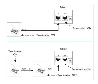
The termination is set in the PM with jumper J4. See "PCB layout diagrams" on page 49 for jumper locations. The factory default setting is for the termination to be set ON. If the PM being configured is 'mid-chain', with both its CAN PORT IN and CAN PORT OUT connectors in use, set the termination to OFF by removing the jumper.
