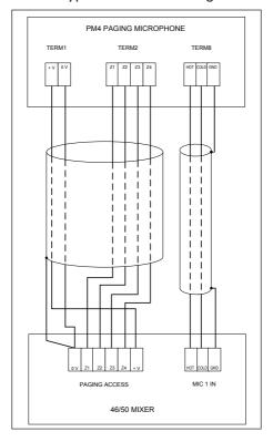
Note in this example that as Zones 5-16 are not in use, no connections need to be made to Z5-Z8 on TERM2, or to Z9-Z16 on TERM4.
