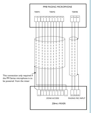
For individual zone paging as described above, the paging mic priority trigger should be selected to 'SW' by moving J5 on each zone sub-board. See page 16 for further information.
