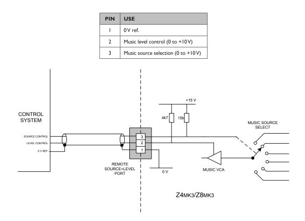
**NOTE:** If the control voltage source is not isolated from the power earth, there is a small risk of creating a 'ground loop' by linking the mixer technical ground (0V) to the ground (0V) of the equipment supplying the control voltages. To minimise this risk, we suggest that all pieces of equipment be in close proximity, and supplied from the same power outlet.
