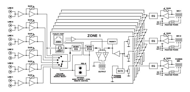
The simplified block diagram above illustrates the basic signal architecture of the Z8MK3. Only the routing and logic for one zone output is shown. The architecture of the Z4MK3 is identical, the only difference being the number of zone outputs.
