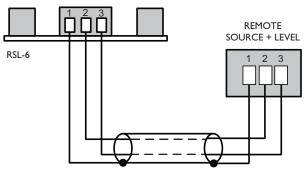
REMOTE SOURCE & LEVEL CONTROL WIRING
