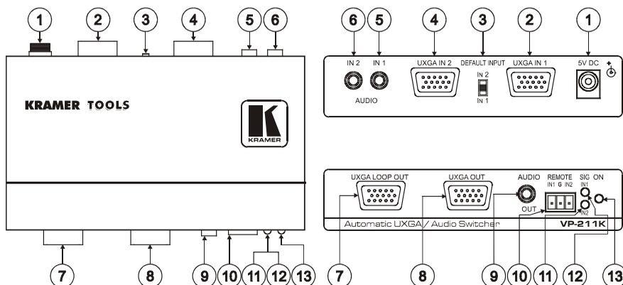
Figure 1: VP-211K Automatic UXGA / Audio Switcher
