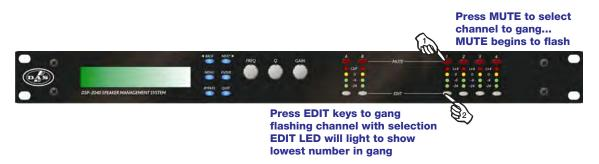
Press a MUTE key to choose the output to gang – its LED will begin to flash, and an EDIT key will illuminate to show which output it is currently ganged with. To change this selection, just press another EDIT key, remembering that gangs work from the highest to lowest number. So, to gang outputs 1 and 5, press MUTE 5 then EDIT 1 – the display will show
