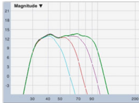
View of DASnet™ with LowPass Filter presets and the Frequency Response Curves
