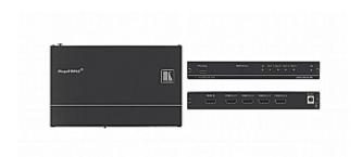
The VM-4UHD is a 1:4 distribution amplifier for 4K@60Hz (4:2:0) HDMI 2.0 signals complying with the HDCP 1.4 content protection standard. The unit takes one HDMI input, equalizes and reclocks the signal and distributes it to four identical outputs.
