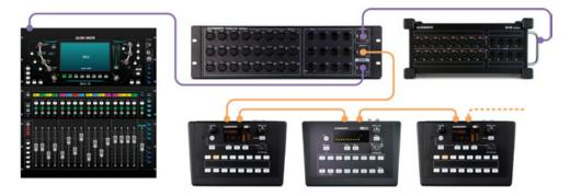
SQ expanded with 2 x DX168 for full 96kHz operation 32 remote inputs + 16 remote outputs
