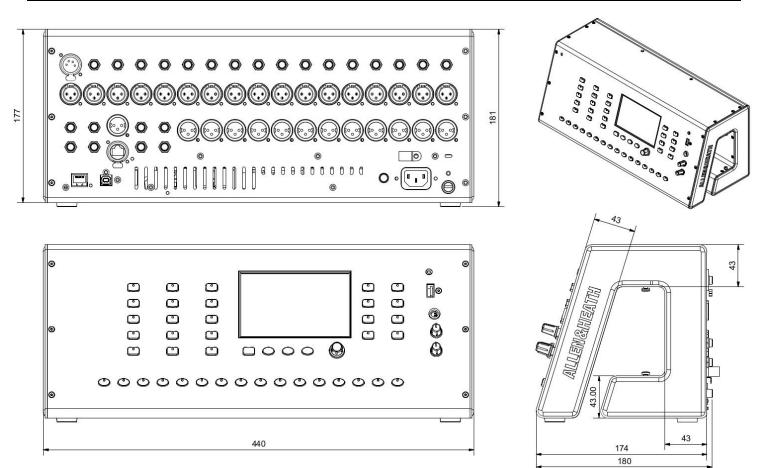
The mixer shall be a compact, rack-mountable digital mixing solution without physical fader strips, but shall include 16 mono and 3 stereo line input channels mixing to 12 mix outputs and 4 stereo rack FX engines, 4 DCA groups and 4 Mute groups. All output mix channels shall contain Insert, Parametric EQ, Graphic EQ, Compressor, and Delay. Signal delays in the system shall be adjustable in Milliseconds.
