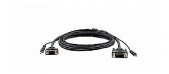
Kramer's C-MDMA/MGMA cable is designed to connect laptop computers to video conference systems that have a DVI input. It adapts the analog pins of DVI-A to a 15-pin HD connector and includes an unbalanced audio cable with 3.5mm mini jacks at each end. Also bundled is a short cable that adapts a 3.5mm mini jack to RCA connectors.
