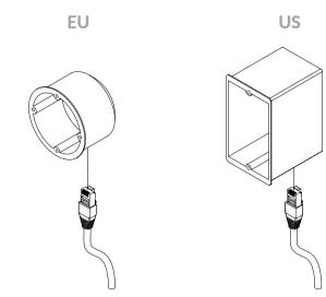
2. Mount the electrical box into the wall.
