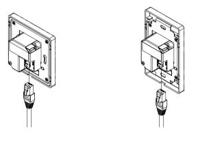
4. Click off the front panel. Screw the Wall-S1 unit into the electrical box. - Put the front panel on - and click it into place.
