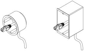
3. Connect the ethernet cable to the Wall-S1 unit.
