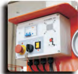
Ground Control With Outrigger LEDs
