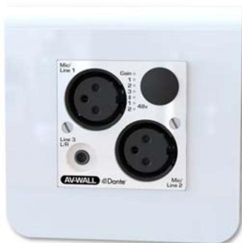
The AV-WALL-DT4i is a compact and cost-effective Dante Mic/Line audio network interface wall plate. It has an internal mixer feature which allows up to 4 lines of audio line mixing. The AV-WALL-DT4i allows for Mic pre-amplification adjustments to be performed either remotely or locally and can be adjusted per 1dB step. The AV-WALL-DT4i is PoE, therefore you only need one Cat5e/6 cable to connect the power, control and transmission.
