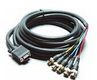
Kramer's computer graphics video breakout cables are constructed of 5 mini coax cables with a molded 15-pin HD (M or F) on one end and 5 BNC (M or F) on the other. They convert between the two most common cabling formats used for routing computer graphic video signals, 15-pin HD, and 5 BNC.
