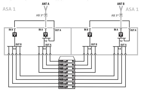
\* AB-3 antenna boosters are only required for longer antenna cables (from approx. 10 m).
