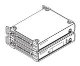
Stack the devices so that the recesses of the stacking elements completely engage with each other.
