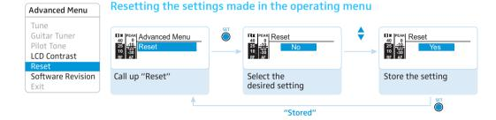
When resetting the settings made in the operating menu, only the selected settings for the pilot tone and for the frequency bank "U" remain unchanged. For an overview of the factory-preset default settings, refer to the supplied frequency information sheet.
