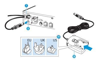
Only use the supplied NT 2-3 or NT 2-1 mains unit. It is designed for your receiver and ensures safe operation.
