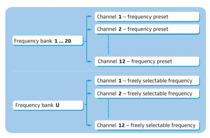
Each of the channels in the frequency banks "1" to "20" has been factory-preset to a fixed frequency (frequency preset).
