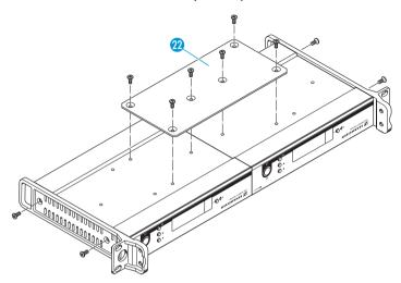
Secure the jointing plate **10** to the receivers using six recessed head screws (M 3x6).
