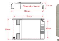
A9920500 3AP LED 3-way serial connection box A9920501 6AP LED 6-way serial connection box
